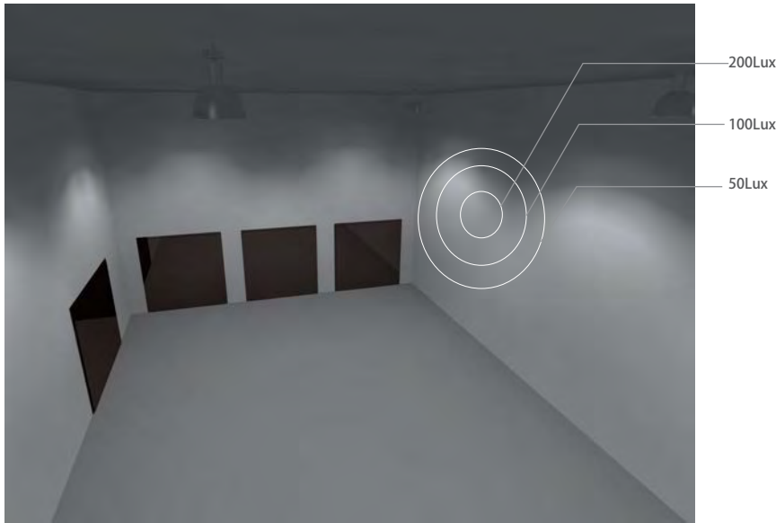
Industrial Area / Storage Building / Ground Floor / Storage / Workplane 5 / Isolines/Perpendicular illuminance (adaptive) Workplane 5 / Isolines/Perpendicular illuminance (adaptive)
